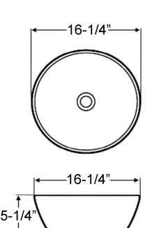
Dimensions of fixture are nominal and may vary within the range of tolerances established by AMSE Standard A112.19.2.2013 Dimensions and specifications subject to change without notice.
